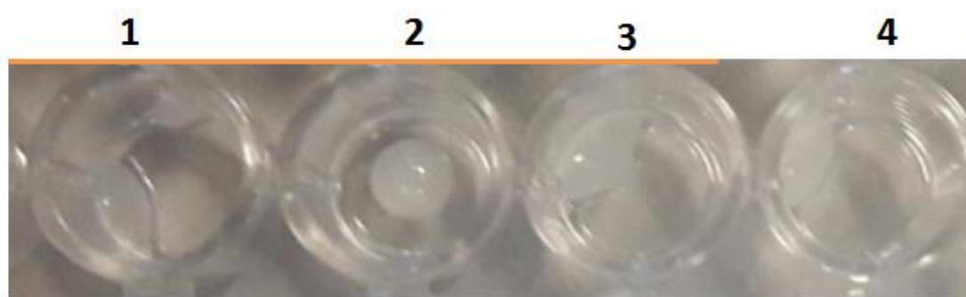
Figure 14. Drop collapse determination test 1, positive control result Triton X-100 (0.1 %); 2, negative control results deionized water; 3, result of TLB 504 strain; 4, result of TLB 506.
